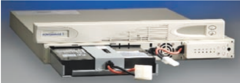
Powerware 5115 RM shown with front cover removed and battery sliding out.
